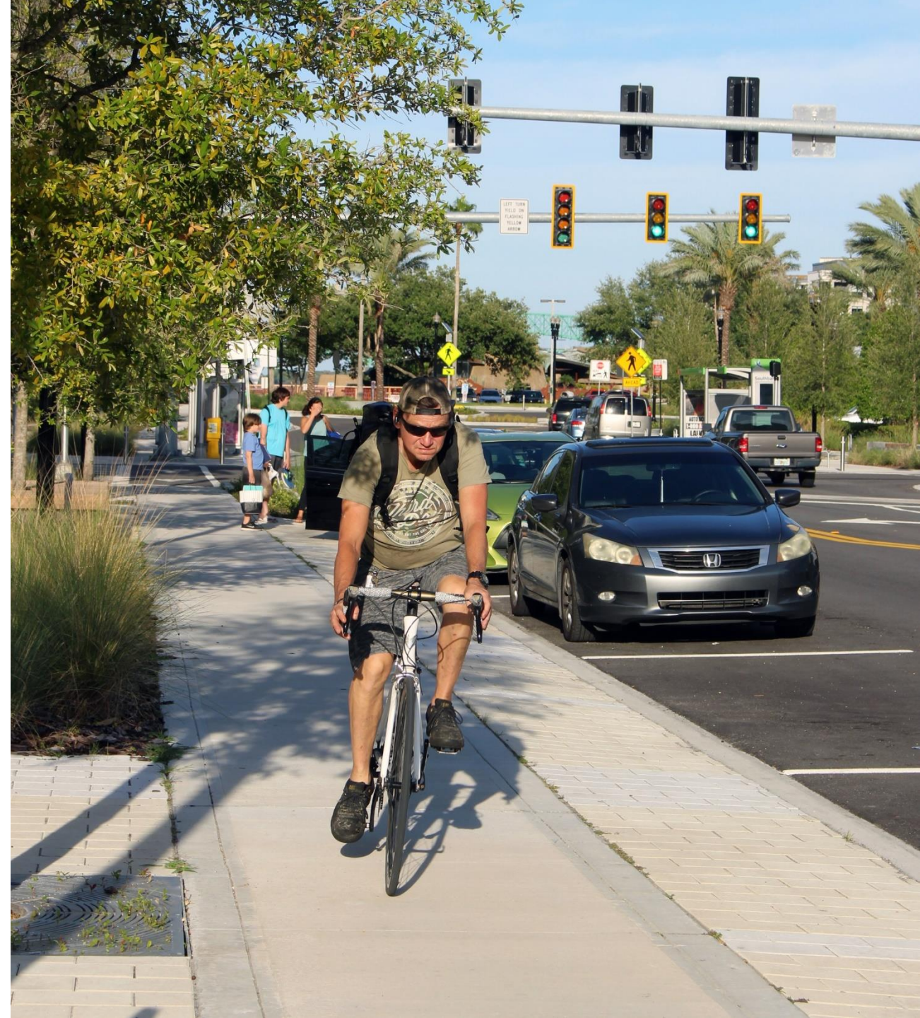
Image #6: Protected and defined bike lanes in each direction, with clear 'step-strips' for on street parking and separate pedestrian streetscape walking and seating areas.
